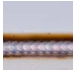
With SFI (spatter-free ignition)
