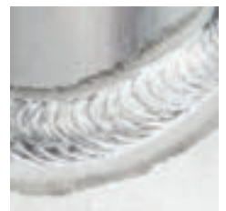
Without SFI (spatter-free ignition)
